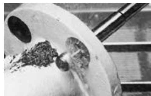
Spindle with coolant through (CT).
