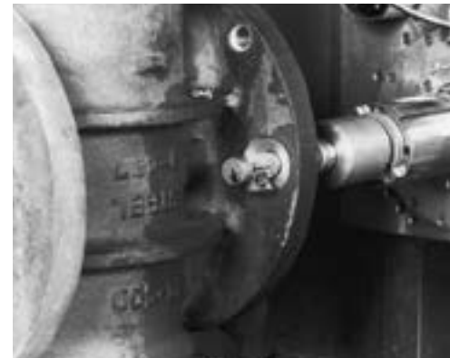
Back spotfacing large valve body.
