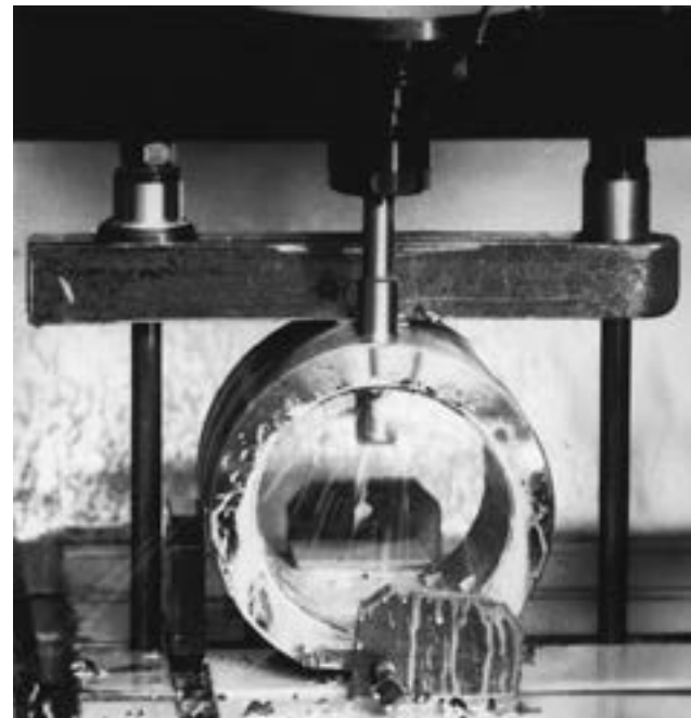
Back spotfacing with coolant through the spindle.
