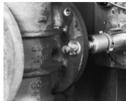
Back spotfacing large valve body.
